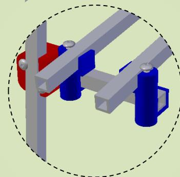
The joiners that the track sits in are upside down with the bolt on the outside of the track and the bolt pointing down.
