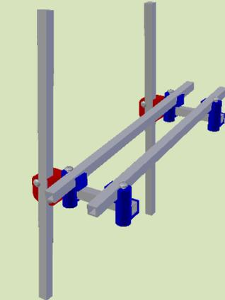
Attach two tracks to the extensions using blue joiners.
